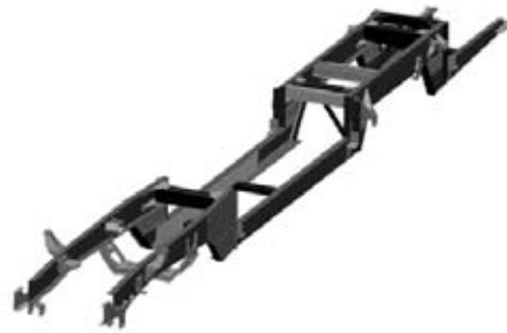
Figure 2. Modified main frame rail
