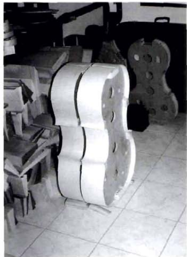
CSELLŐ SABLON ÖLDALLAL LA FORMA DEL VIOLONCELLO CON LE FASCE CELLO MOULDS WITH THE RIBS IN PLACE
