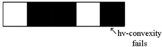
Figure 5.3 If a black pixel occurs behind a 1-to-0 transition, the hv-convexity condition fails
