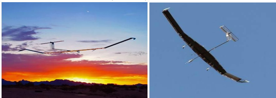
9.3. ábra. Airbus Zephyr 8 HAPS UAV [2.77, 2.78].
