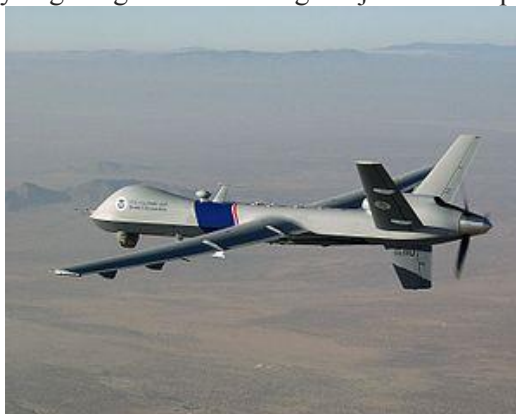
2.31. ábra. General Atomics MQ-9 Reaper (Predator B) UAV [2.41].
