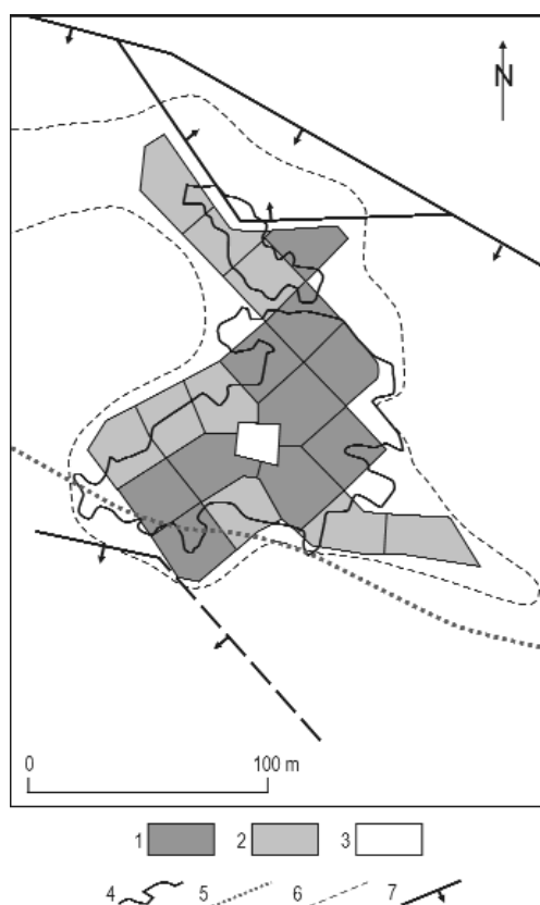
Figure 53. Resource estimation map of the Nyíres-kút III lense. Polygon method (1958 and 1993)
