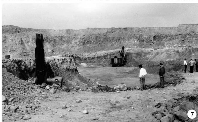
7. Open pit of lense No. XI in 1970. The central part of the lense. In the lower part red bauxite, above it middle Eocene limestone.
