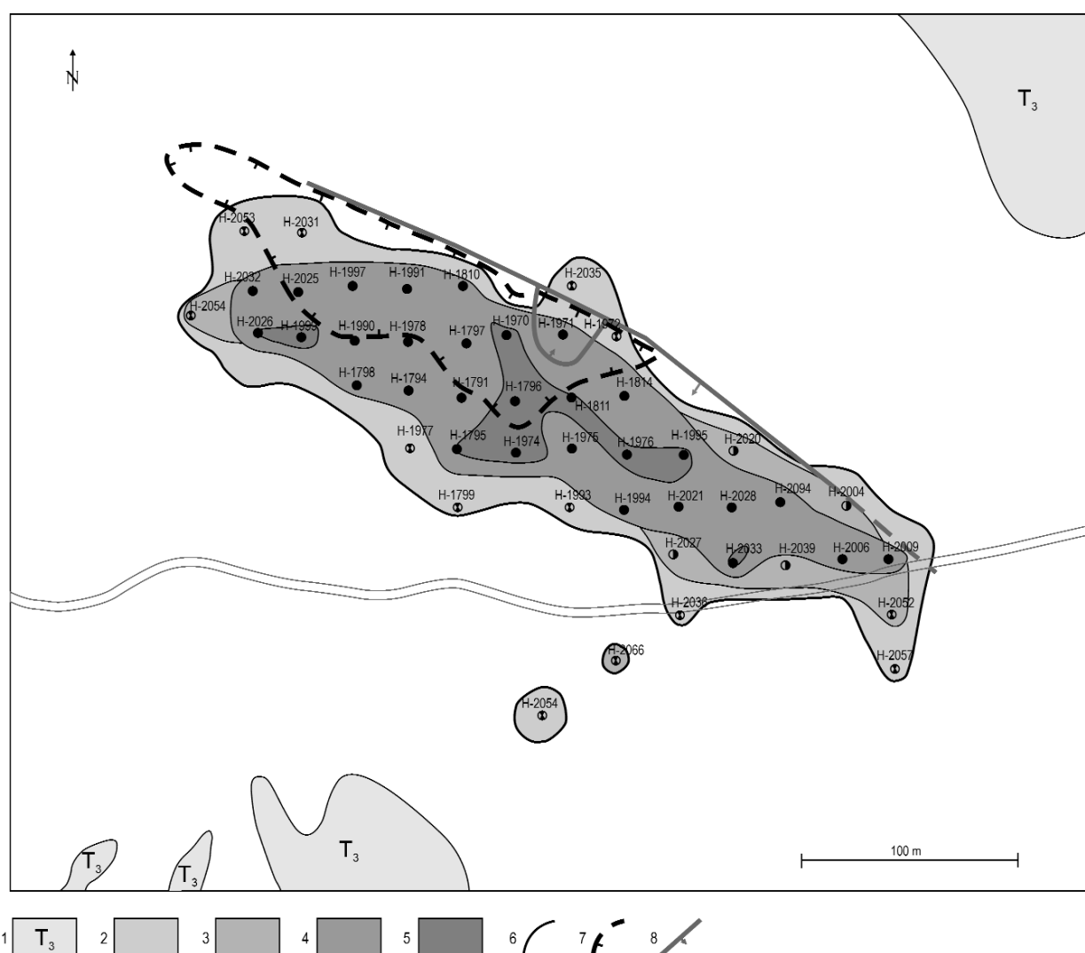
Figure 43. Mining geologic map of the lense No. XVI
