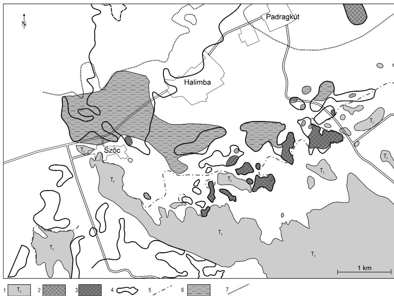
Figure 4. Distribution of the middle Eocene grey lignitic clay in the Malom-völgy deposit and in the southern part of the Halimba Basin
