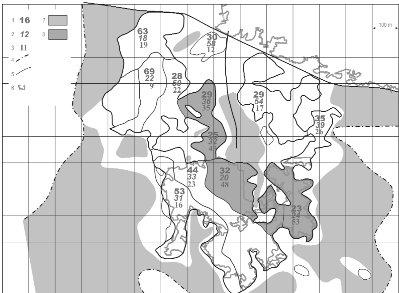
Figure 16. Percentage of the thickness of the three bauxitic rock types in the southern part of the Halimba deposit.
