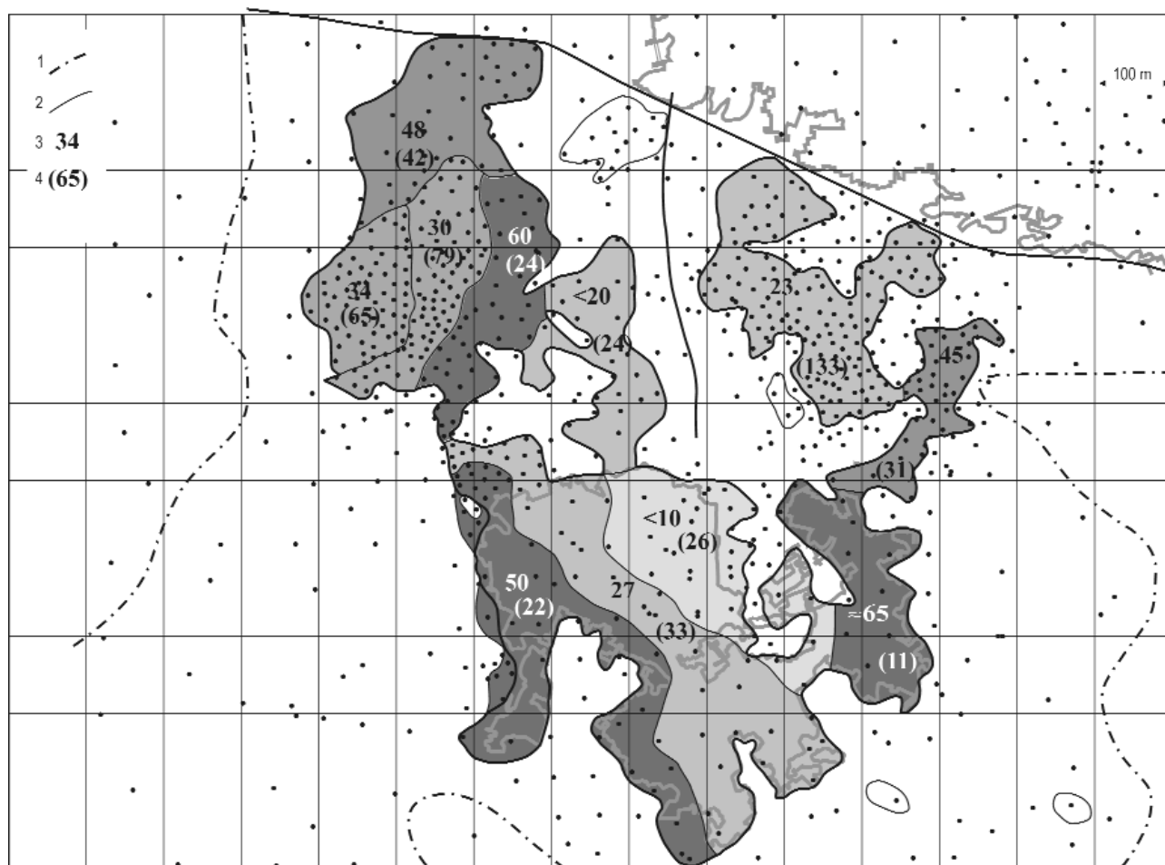
Figure 12. Ranges of influence of the bauxite thickness calculated from the variograms in the southern part of the Halimba deposit 1 — contour of the bauxite sequence, 2 — contours of the sectors, 3 — ranges of influence (metre), 4 — number of boreholes involved into the calculation
