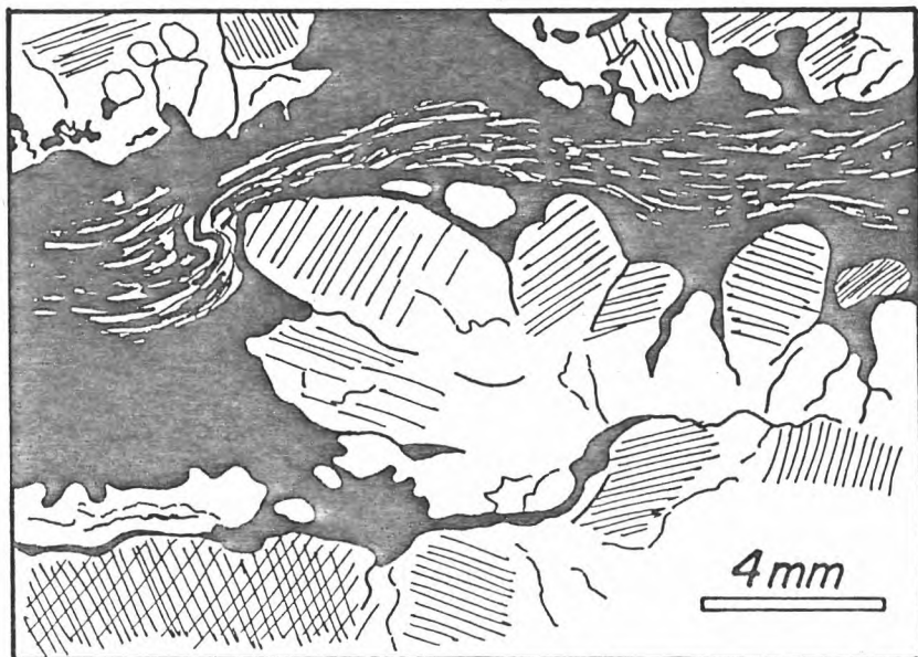
Fig. 1.- Thin section aspect of calcitized pseudodiapiric nodules. Sometimes relict gypsum precursors can be seen.
